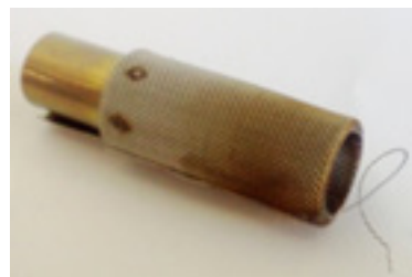
Fig. 3b. A burr on the screen
