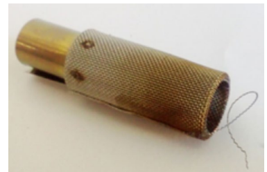
Fig. 3b. A burr on the screen
